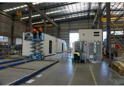
+ Transportable: built and tested off-site
