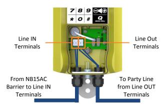
Although the VoiceCom Phone can be directly installed in place of an IS2000 Telephone, it is important to note that the IS2000 Telephone and the VoiceCom Phone are not compatible when installed in the same party line configuration. That is a VoiceCom Phone cannot be on a party line with an IS2000 Telephone.
