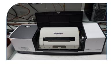
The new FTIR instrument, a Shimadzu IRSpirit with Specac Pearl sampling attachment (Figure 2) is a compact modern instrument that is reliable, precise and easy to use.
