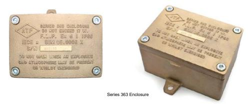
The Enclosure has been certified as explosion protected category Ex d for Group I gases (Methane) with a maximum surface temperature of ≤ 150°C as determined by the original test when operating at maximum power dissipation.
