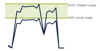
By using our PFC equipment, the total amount of electrical demand is reduced, by reducing or eliminating wasted reactive power (kVAr), seen as the green portion in the above graph.
