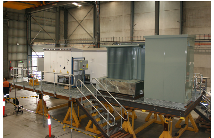
Power conversion skids being manufactured in Ampcontrol's workshops
