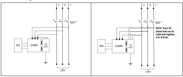
NOTE: When the CCM is fitted the IP relay will measure a parallel combination of the cable resistance and the CCM load module resistance. The "Insulation Test" levels will need to be reduced to the  $0.5M\Omega$  setting (or below) to ensure correct operation. This trip does not correspond to a  $0.5M\Omega$  for the cable insulation.
