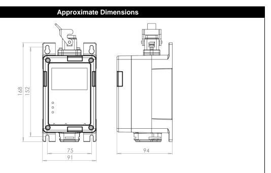
\*Note: While mounting points remain the same, the additional space required by the GG2 Display/Detector assembly must be taken into account. The remote head assembly will require a bracket modification to mount the detector.
