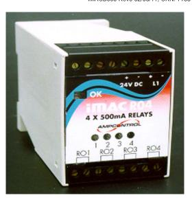
**Fast flash** (continuous 0.3s apart) if the L1 line is open or short-circuited. Or polarity to module is incorrect.
