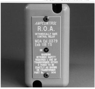
The loop resistance of the circuit will be 100 ohms plus the resistance of the cable. When the start button is pressed the contacts short out the 100 ohm resistor and provided the cable resistance is less than 45 ohms the relay will energise. When this occurs the normally open and normally closed contacts change state. The LED on the front of the module will be illuminated. This indicates a healthy control circuit.
