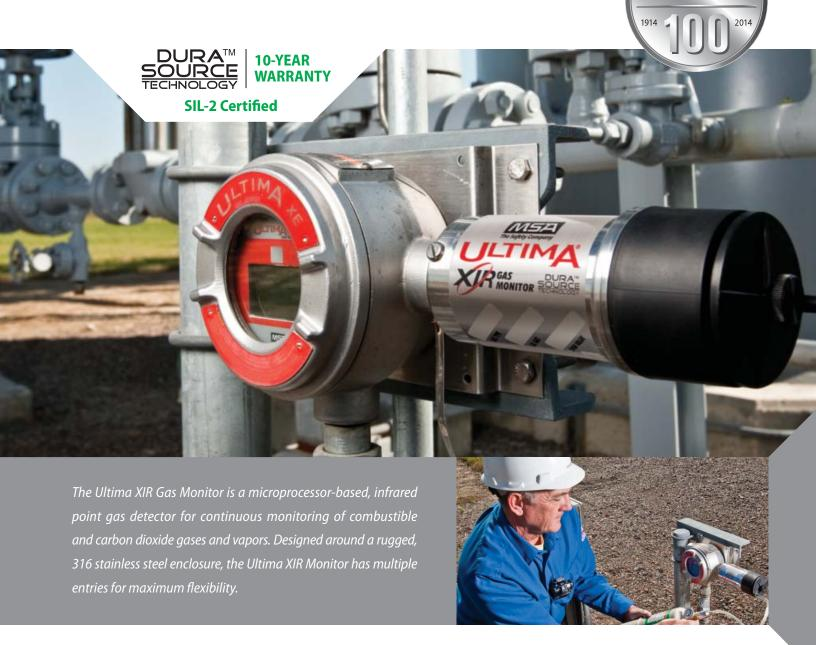
Ultima XIR Monitor operation is based upon dual-wavelength, heated-optics technology providing definitive compensation for temperature, humidity, and aging effects. IR technology offers excellent long-term stability, eliminates the need for frequent calibrations, and reduces overall cost of ownership.
