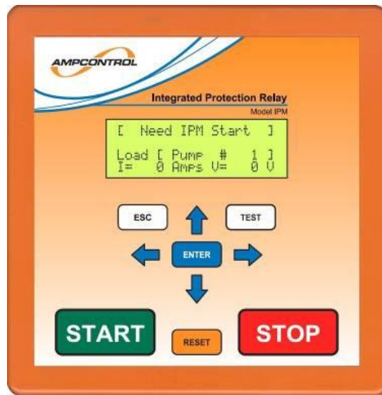
Figure 12.1: IPM Relay Fascia and Display
