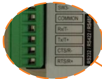
Serial Communications Port Terminals
