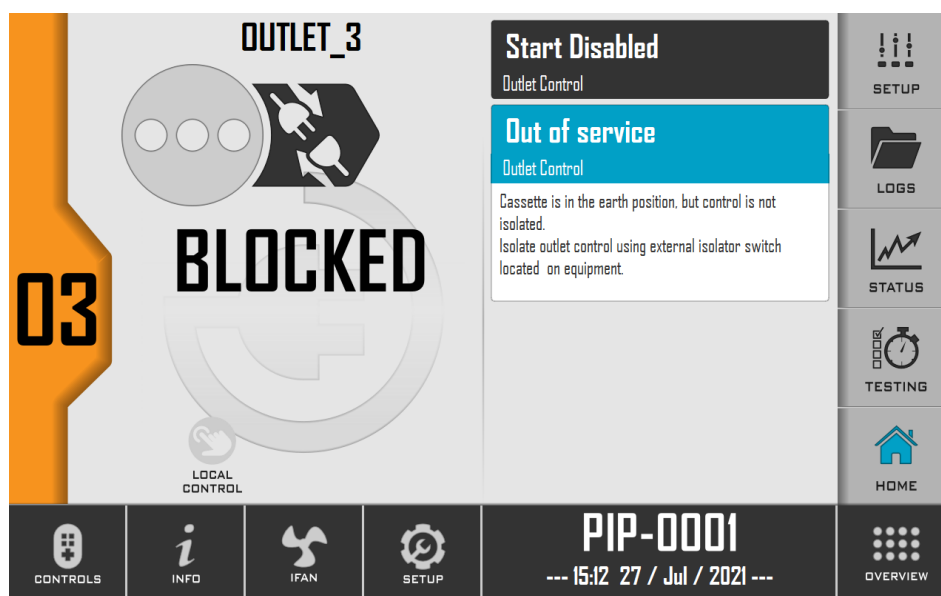
Figure 68: PIP Withdrawable Outlet Home Interface, Outlet Cassette in Earth Position – Actuator Not Isolated
