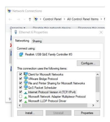
Select "Use the following IP address" and enter an IP address in the same subnet as the vi. Rockstarter. If you are not sure then set the Rockstarter and the laptop to the same IP details as this in the image below.
